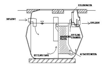
Figure 2.8. Typical cross-sectional drawings of prefabricated septic-tank anaerobic filter type systems (Kazmi A. A. 2003)
