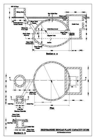
Fig 3.12 Drawing of a 4 cum biogas plant – Deenbandhu Model
