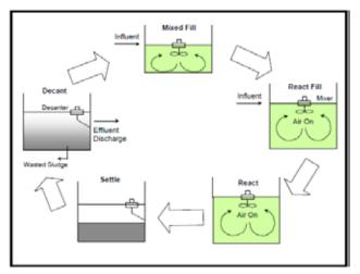
Figure 2.37. A Typical Cycle of Sequencing Batch Reactor (USEPA 2000)
