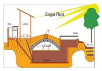
Fig. 3.10 A section of family size biogas plant of Deenbandhu Model (Source: Grassrootindia.com2013)
