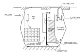
Figure 2.12. Typical cross-sectional drawings of package anaerobic filter-contact aeration system (Kazmi. 2003)
