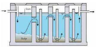
Fig. 2.28. Anaerobic Baffled Reactor; (Source: Morel & Diener 2006)
