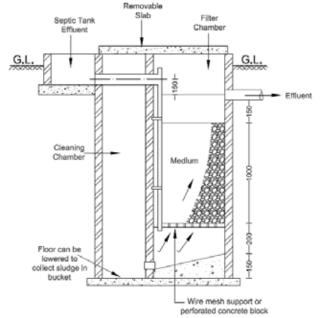
Figure 2.9. Typical cross-sectional drawings of conventional septic-tank anaerobic filter type systems (IS 2470: Part 2: 1985)
