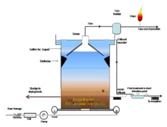
Figure 2.31. Schematic Diagram of UASB based plant (Source Kazmi A. A.2003)
