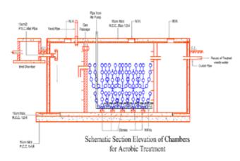
Fig 2.35 Schematic diagram of settling –contact aeration system
