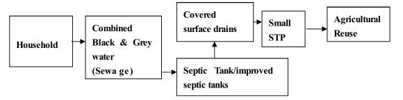
**Option-7: (Partly Sewered sanitation using small bore sewer)**
