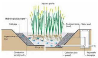
Figure 2.25. Horizontal flow constructed wet land: Tilley et al. (2008)
