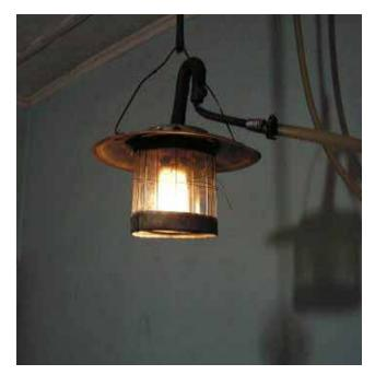
Fig. 3.14 Biogas being used as lighting through mantle lamp
