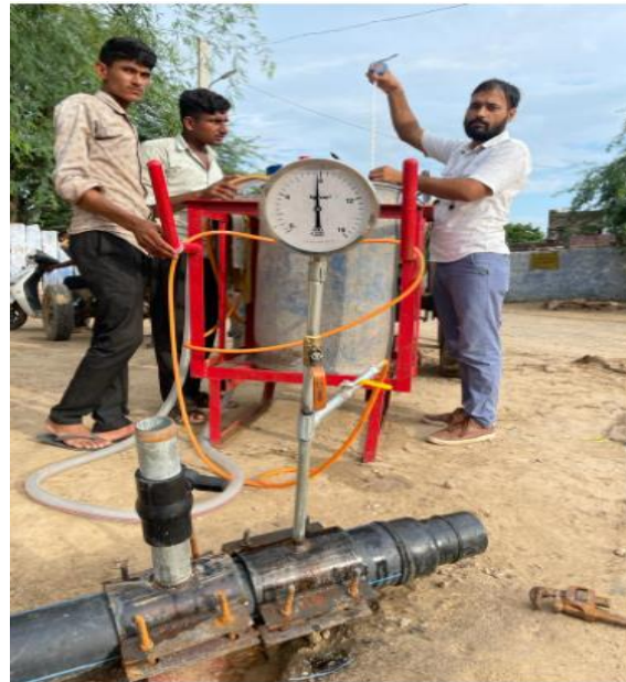
HDPE Pipe Testing
